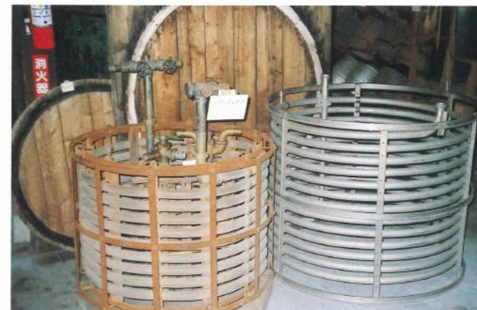
15 Jakan, an apparatus with a long coiled pipe that is heated to 60 degrees, and through which newly distilled sake is sent for the disinfecting process. Displayed in the 300-year-old Matsuiya Sake Manufacturing grounds.
