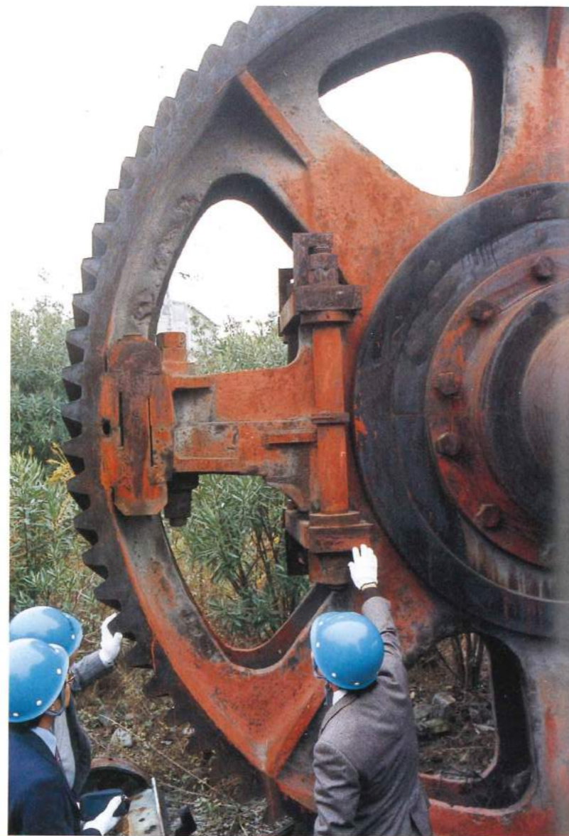
58 The cogwheel has a diameter of 4.2 meters and weighs 65 tons. It was used from 1937 to 1961, and is now preserved at Chubu Kohan Company.
