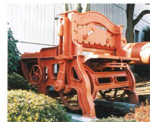
91 The American-made cutter, made in 1890, for cutting rolled paper into sheets, used at the Iriyamase factory of Fuji Paper Manufacturing Co..
