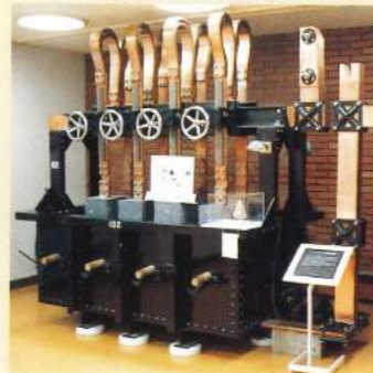
Aluminum electrolysis tank in the Oomachi Energy Museum
