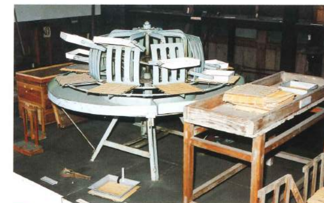
85 Semi-automatic seaweed thinning machine, built in 1955 and displayed at the Toyohashi Folklore Museum.
