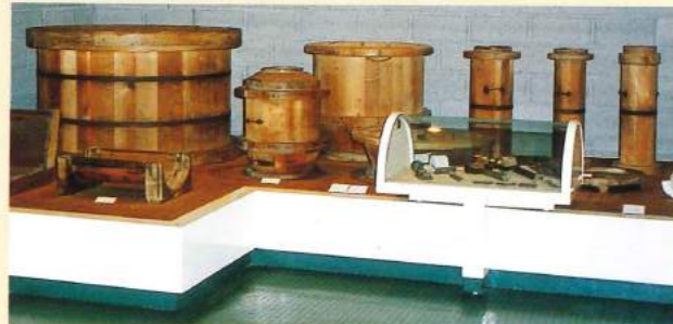
Wooden molds to make earthenware pipes, Tokoname City Folk Museum
