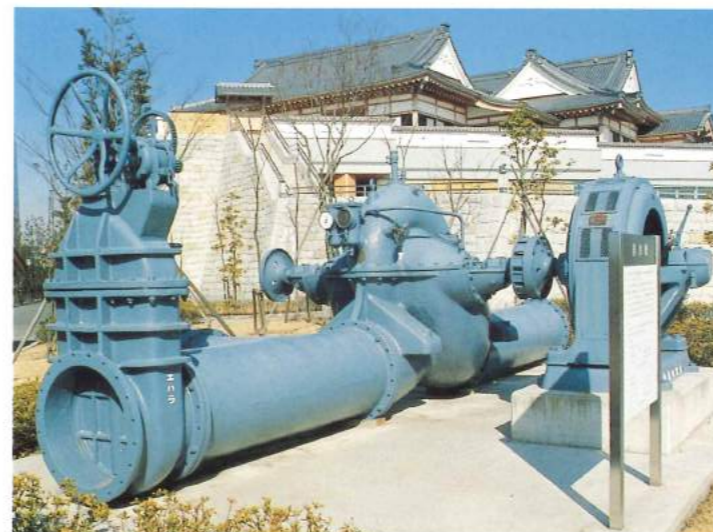
84 Volute pumps at the Fukue Drain Pump House, built in 1927, released 1.8 tons per minute of water into the Ibi River. These were in operation for 56 years.
