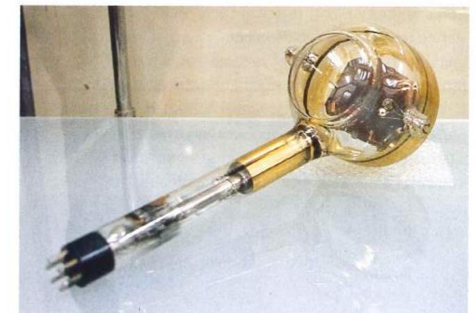
53 Takayanagi's first iconoscope, which employed his theory of transforming light from an image into electrical signals through the use of a condenser. He was successful in 1935 in using the iconoscope to capture an outdoor image onto a cathode-ray tube. Displayed at Takayanagi Memorial Museum.
