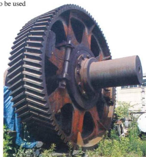
58 The cogwheel has a diameter of 4.2 meters and weighs 65 tons. It was used from 1937 to 1961, and is now preserved at Chubu Kohan Company.
