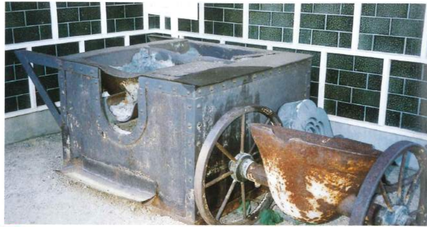
61 Pot for removal of copper slag from cooled raw lead, used in the purification of lead. This machine was installed in 1924 at Kamioka Mine, and was used continuously up through 1968.
