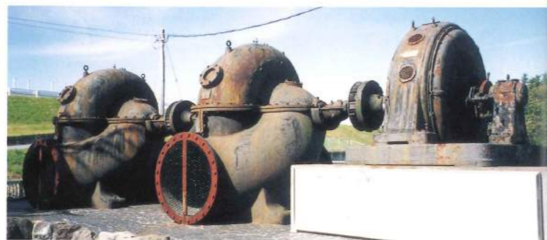
82 Volute pumps, made in 1928, releasing water into the Nagara River at 9 tons per second, were in operation for 55 years.
