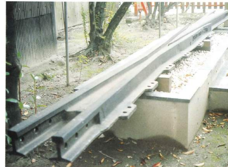
56 The high-manganese alloy crossing rail, built in 1948 by Daido Steel for the Chuo Line of Japan National Railways and laid in Ochanomizu Station.
