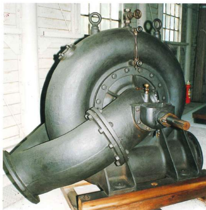
39 Oldest existing Inokuchi-type volute pump in Japan, built in 1912.
