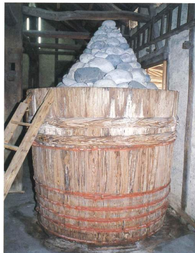
17 A view of the inside of the fermentation cellar for Hatcho-Miso in the North Cellar of Maruya Company. The wooden Miso tub holds 6 tons of ingredients, for a total weight of 10 tons with the stones piled on the lid.
