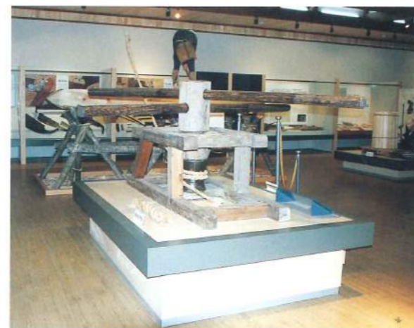
89 The Kagurasan, an apparatus used in the Hida region for hoisting the wood onto and off of the rafts, much like today's winch.
